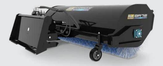
The hydraulic rotary broom comes ready with everything you need including hydraulic hoses, flat-faced couplers, and an electric selector valve, and wire kit. Hooked up and ready to go, the broom's direct motor drive requires 12-20 GPM of hydraulic flow to turn the 26" diameter poly/steel wafers.
